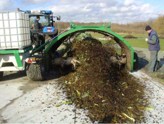
Compost pile with compost turner and tractor with water tank: compost slurry is turned for aeration and moistening of compost - ILVO
